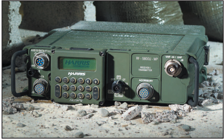
Figure 1. HF tactical radios provide long-range communications capabilities using frequencies from 1.6 to 30 MHz. (Photo courtesy of Harris Corp.)
